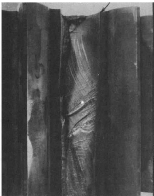
Fig. 4 Spur pinion failure. Tooth-bending fatigue with origin at root radius of loaded side at one end of the tooth. Original magnification at 0.6x
