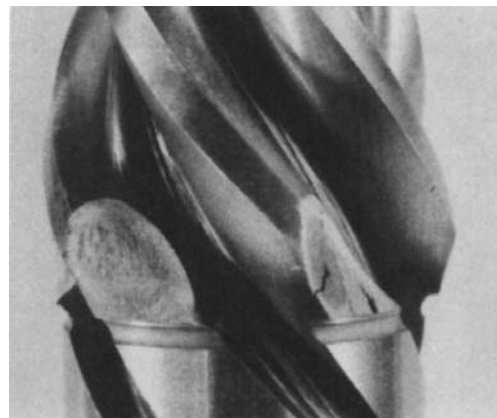
Fig. 31 Tooth chipping resulting from impact of a foreign object within the assembled unit
