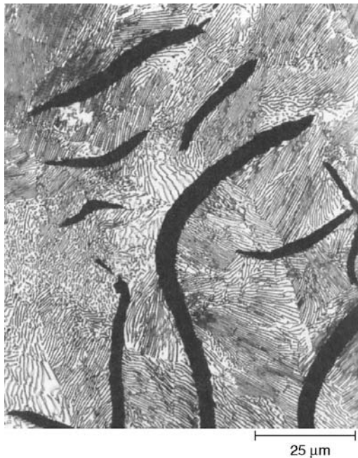
Fig. 32 Flake graphite in a pearlitic matrix in a class 30 as-cast gray iron
