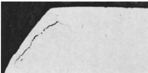
Fig. 25 Subsurface cracking that subsequently resulted in spalling at a gear-tooth edge. Unetched section of a carburized AMS 6260 steel gear tooth. Cracking initiated in the transition zone between the carburized case and the core. Original magnification at 500 \times
