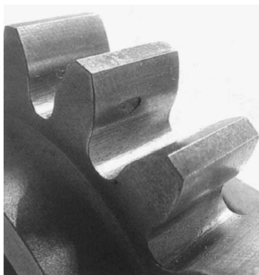
Fig. 12 Gear with arrow-shaped surface-origin pit. Source: Ref 4
