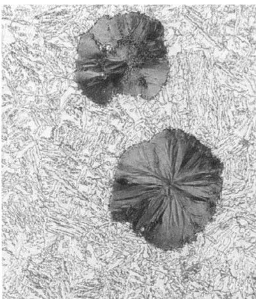
Fig. 35 Austempered ductile iron structure consisting of spheroidal graphite in a matrix of bainitic ferritic plates (dark) and interplate austenitic (white)
