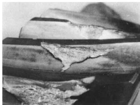
Fig. 23 Spalling of spiral bevel gear teeth. Original pitting low on the active profile gives initiation to a fast and extensive progression of spalling over the top face and down the back profile. This is often called the cyclone effect. Original magnification at 0.25\times
