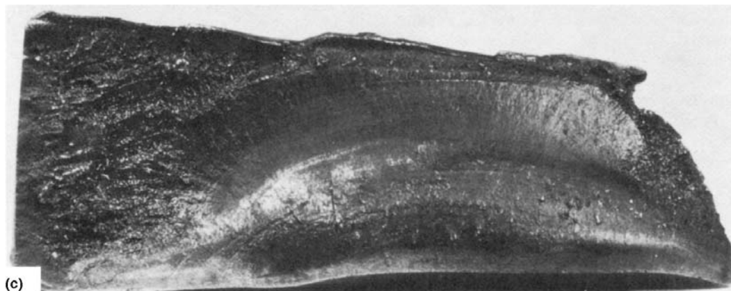
Fig. 51 2317 steel bevel pinion that failed by fatigue breakage of teeth. (a) Configuration and dimensions (given in inches). (b) View of area where two teeth broke off at the root. (c) Fracture surface of a broken tooth showing fatigue marks
