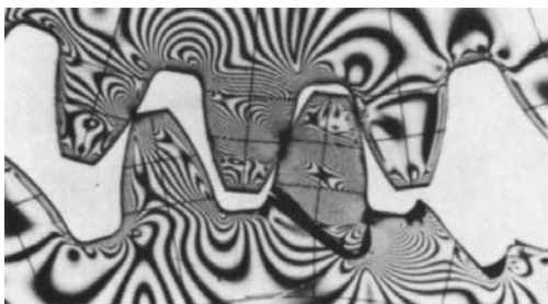
Fig. 2 Photoelastic study of mating teeth indicates the shift of the zero-stress point during crack propagation until final fracture reaches the opposite root radius. At the same time, deflection of the tooth allowed the adjacent tooth to pick up the load
