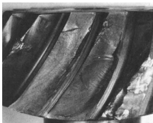
Fig. 1 Spiral bevel pinion showing classic tooth-bending fatigue. The origin is at midlength of the root radius on the concave (loaded) side. Original magnification at 0.4x
